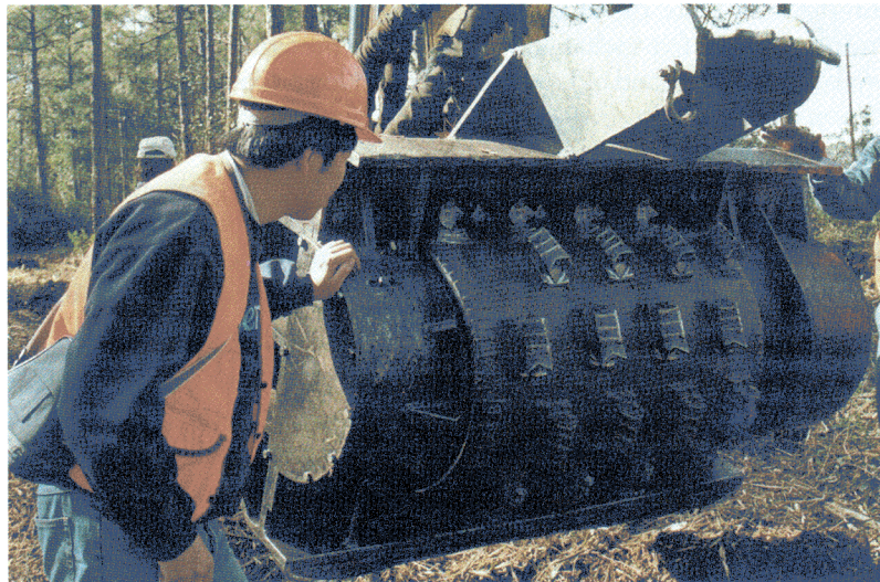
Fig. 1: The Shinn SC-1 boom-mounted rotating drum.
