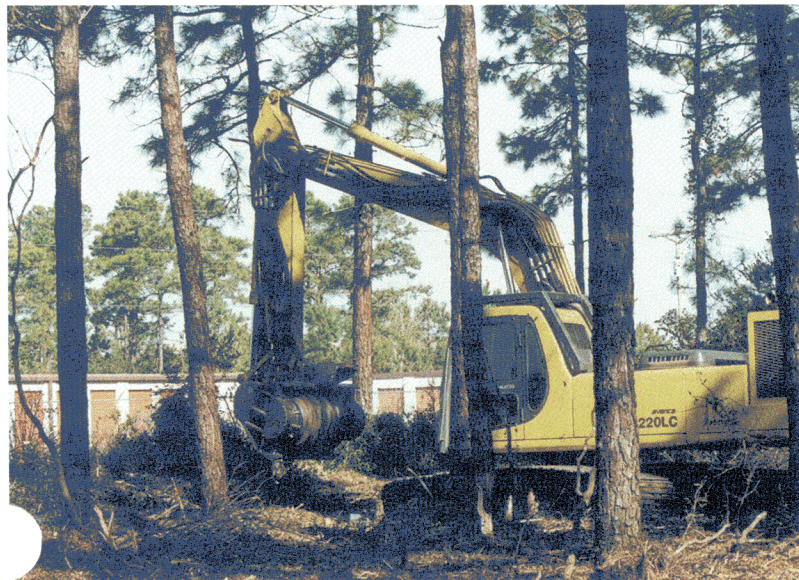
Fig. 2: The Shinn SC-1 head at work on a Komatsu excavator.
