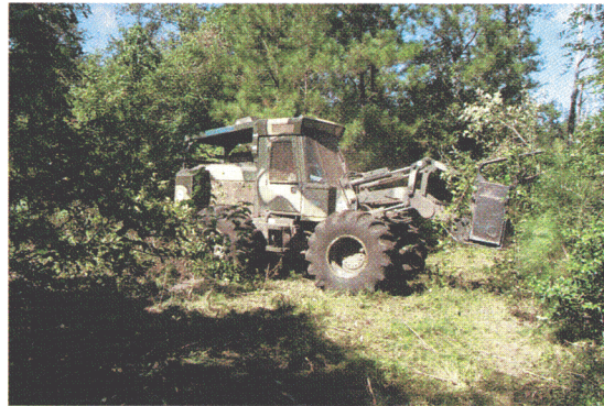
Fig. 1: The Woodgator® mulches vegetation for stand improvement and reduction of wildfire risk.
