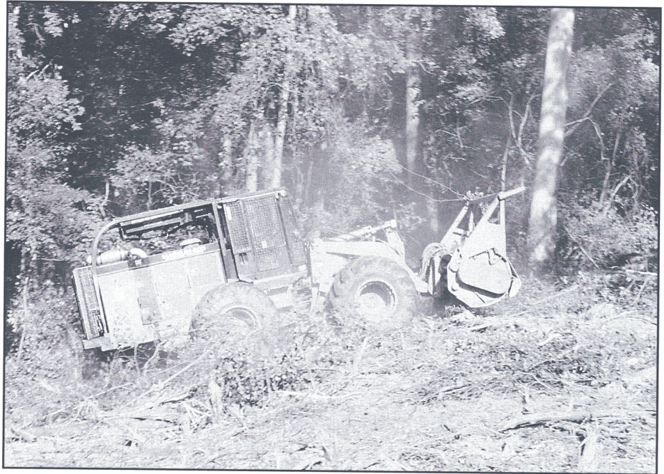
Photo 3: Horizontal shaft machine in operation.
